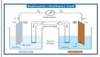
It generally consists of two half cells and a salt bridge. Each half-cell further consists of a metallic electrode dipped into an electrolyte. These two half-cells are connected to a voltmeter and a switch externally with the help of metallic wires.
